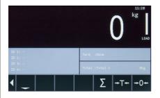
8. If the weight is red, the weighing was not correct. If the indicator does not show zero, a new zero must be set manually. See: 3.4.2
