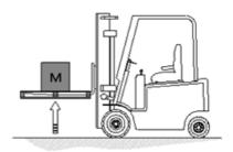
If the arrow turns in the opposite direction lower the forks with a constant speed until the weight appears on the display.
