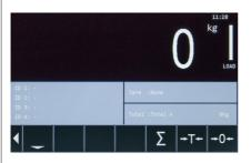
To perform a weighing cycle, pick up the load and lift with constant speed for as long as the yellow arrow keeps blinking in upward direction. If the arrow turns in the opposite direction lower the forks until the weight appears in the display. For detailed explanation see: 3.4.1 step 3-6
