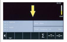
4. If the weighing was done correctly it appears in the display without any messages.
