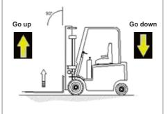
After passing the measuring trajectory the speed indicator will show the average speed of the forks if it was incorrect.
