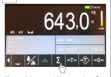
After completing your weighings, press the  $\to \Sigma \leftarrow$  key to save all data on the indicator.
