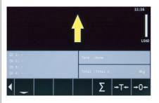
Lift empty forks with a constant speed until the blinking yellow arrow at the display shows you to lower the forks.
