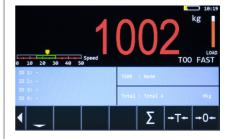
3. Error: **Try constant speed**Try to move the forks faster with a constant speed through weighing trajectory.
