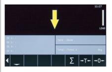
Lower the forks with constant speed until the forks on the display are in their lowest position.
